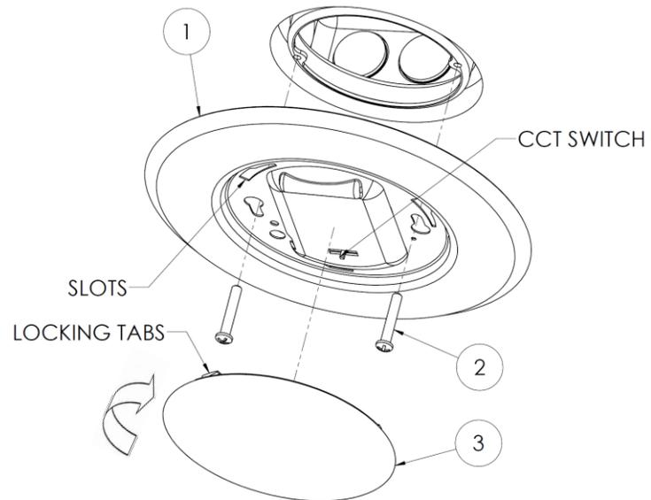
View shown for reference only. Individual models may vary. Note: Mounting hole spacing on SLMF04 will be just 2.75"; SLMF06 will be 3.5" and 4.75"
